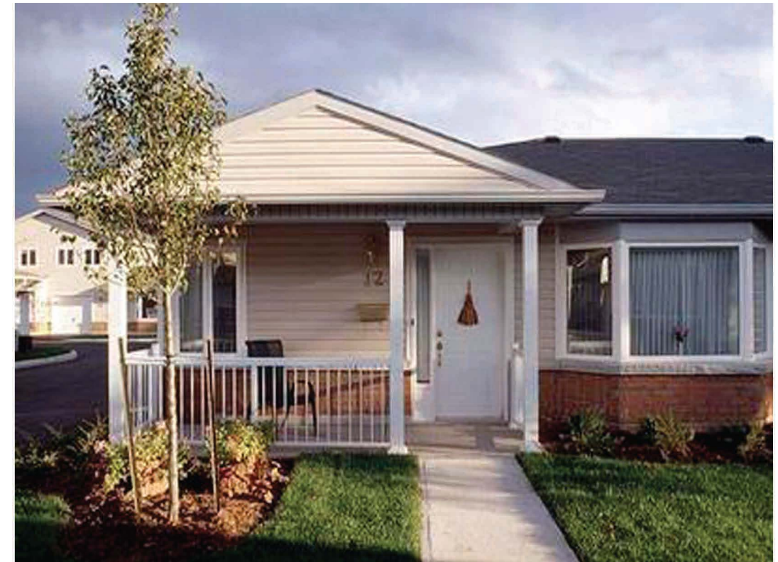
At Woodside Mews, a life-lease community for the elderly, the homes have design features to allow seniors to age in place, such as an at-grade entry.
